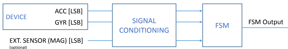
Figure 2. State machine in the LSM6DSOX
