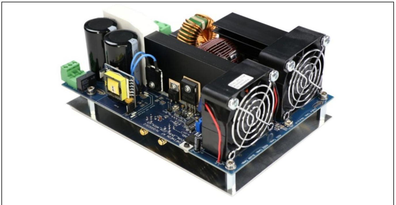
Figure 33 Photograph of a PFC evaluation board, which was used to determine the efficiency measurements shown. This demo board is available to order under “EVAL_2k5W_CCM_4P_V3” via www.infineon.com [18].
