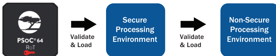
Figure 5: Boot time security requirements - Secure Boot flow
