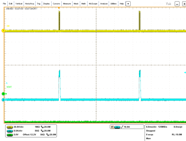
Figure 22. Hiccup in persistent short-circuit
