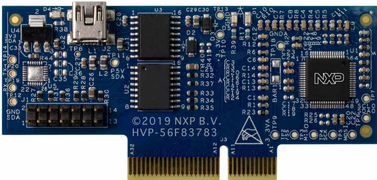
NXP HVP-56F83783: The High-Voltage-Development Platform is a hardware and software rapid prototyping toolset for evaluating high-voltage motor control and power conversion designs and algorithms.
